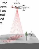
systems. "Small footprint" means that the laser pulse diameter at ground level ranges from 15 to 90 cm.
