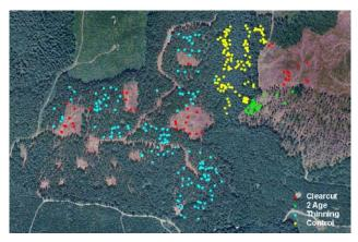
Survey checkpoints used to evaluate bare-earth surface model accuracy
