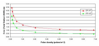
Error in Lidar-derived tree height measurements increases as the pulse density decreases.
