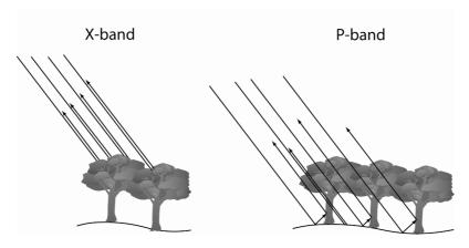
Figure 3-9. Short wavelength X-band RADAR energy reflects from canopy surface while long wavelength P-band energy penetrates through canopy and reflects from stems and terrain surface Adapted from Moreira et al. (2001).
