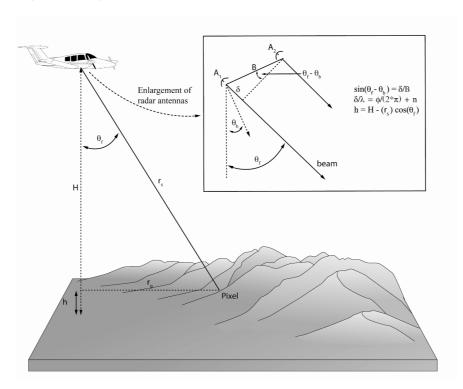
Figure 3-10. Geometry of RADAR interferometry. Adapted from Mercer (2004).
