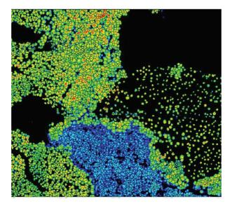
Figure 3-6b. Individual tree-level segmentation of LIDAR canopy height model via morphological watershed algorithm (color-coded by height: blue =  $20\,$  m, green =  $30\,$  m, yellow =  $40\,$ m, red =  $50\,$ m; black lines indicate boundaries of segments; black areas indicate areas with no tree cover). (See also color plate 3-6b on p. CP4)
